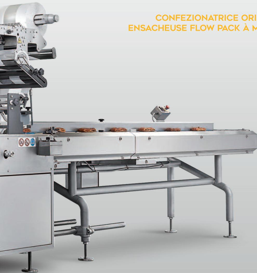
Electronic flow pack machine for modified atmosphere packaging (MAP) guaranteed by the box motion system. Suitable for wrapping bulky products, such as panettoni or multipacks, and is also suitable for applications using thick materials or films.
